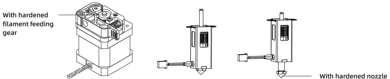
Twist off the standard nozzle by wrench and replace it with the hardened steel nozzle. After changing the nozzle, please do z-calibration again.
